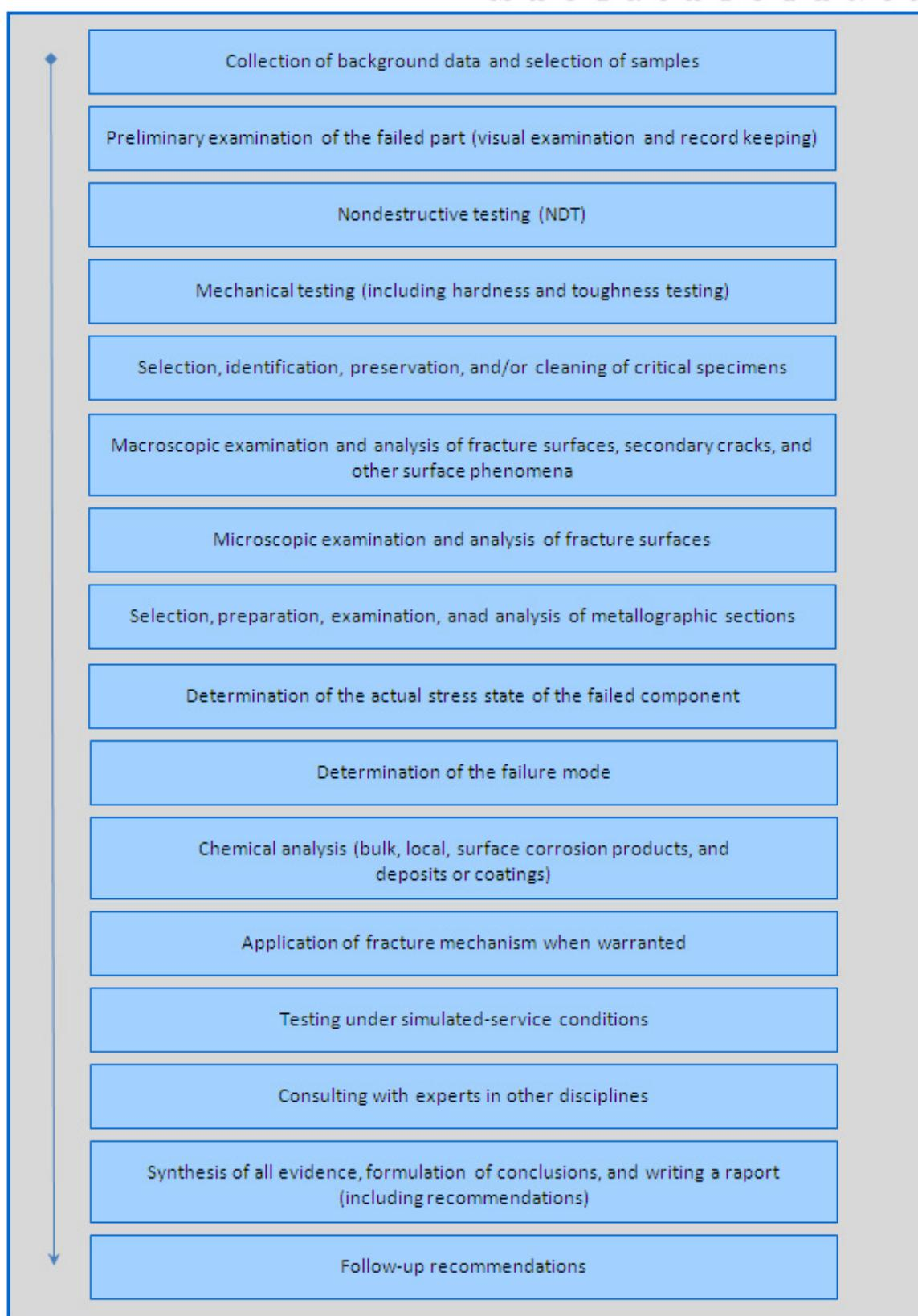
Source: How to organize and run a failure investigation / Daniel P. Dennis / Stages of a failure analysis
