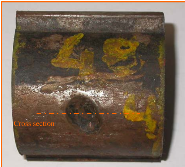
Fig.1: Received tube sample with local wall thinning on furnace side. Location of cross section as in fig. above.
