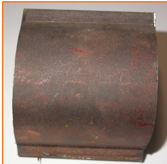
Fig.2: Same tube sample seen from insulation side.
